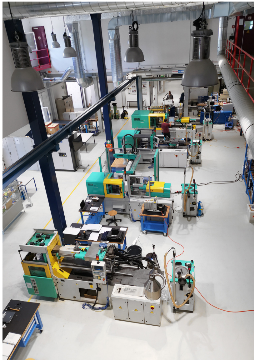
Fig. 2 Laboratory for Plastics and Ceramic Injection Molding at the Institute for Applied Plastics Research (iRAP) in Fribourg. Beside injection moulding, iRAP is active in compounding and recycling, composite materials, material characterisation, surface treatments and nanotechnology. The institute has specific expertise and equipment for Ceramic Injection Moulding and supports industrial partners in the development of innovative products, processes and solutions (Courtesy HEIA-FR /HES-SO)
