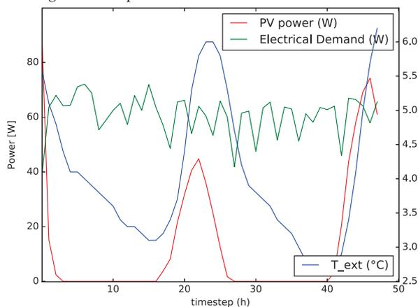
Fig. 3 Example of algorithm predicted data for 48 hours. The daily variation of the solar panel production and outside temperature are determined by weather forecast and the building energy needs is computed from the physical model. In this example the users power need is limited to the devices standby mode (60 W continuously)
