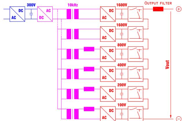
Fig.2 Schematic diagram of the MAGY modulator
